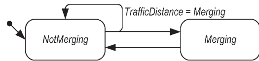
Fig. 10. State transition diagram depicting the formal model’s behavior for the presence of merging traffic ( Traffic ).
