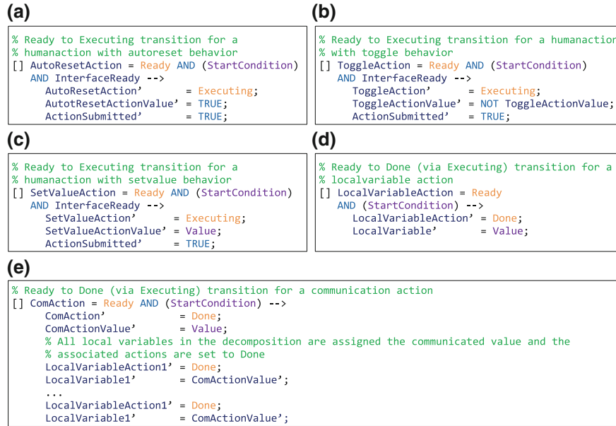
Fig. 13.10 Patterns of SAL transitions used for an action to transition from Ready to Executing and/or Ready to Done with an implied execution in between. a The pattern used for a humanaction with autoreset behavior. b The pattern used for a humanaction with toggle behavior. c The pattern used for a humanaction with setvalue behavior. d The pattern used for a localvariable action. e The pattern used for a communication action. Note that LocalVariable1 – LocalVariableN represent local variables in a com decomposition that received the value communicated. Further note that in c , d , and e , Value is used to represent a variable or specific value from the XML markup
