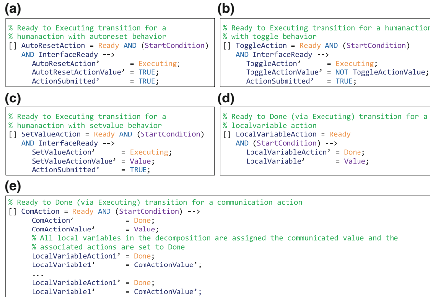
Fig. 13.11 SAL transition pattern used to handle action Executing to Done transitions
